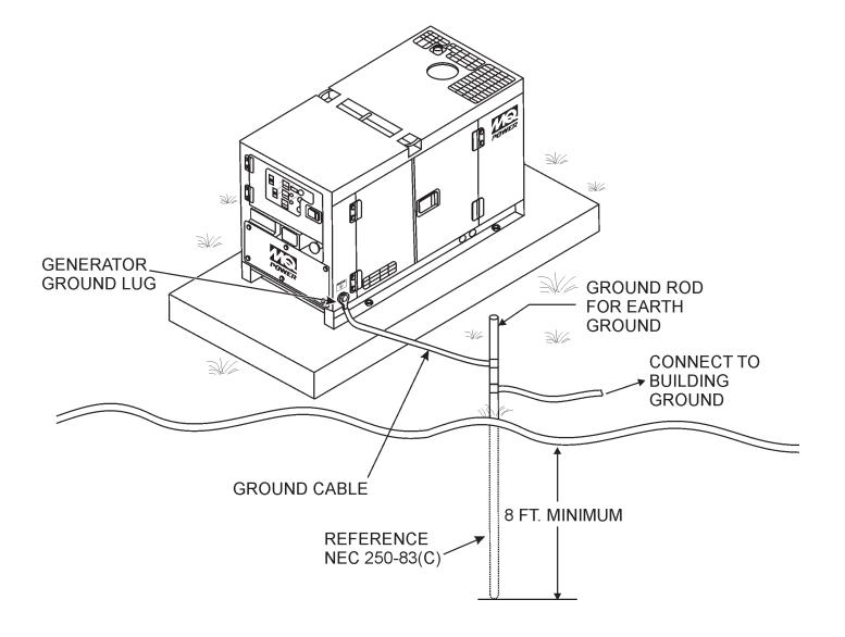
Figure 4. Typical Generator Grounding Application
